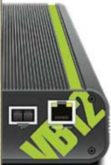
**VB12** is the most portable broadcast monitoring and measurement platform available. Featuring both optical and electrical GigE Ethernet inputs, separate management port and both an ASI input and output, the VB12 has the widest range of built in interfaces in any portable product in the industry.
